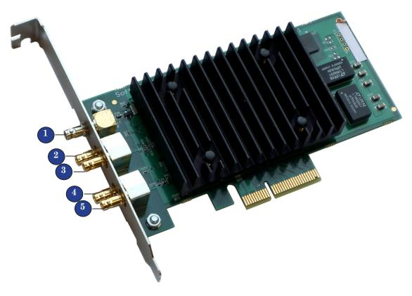
HD-BNC connectors are used to plug signals sources/receivers to board:
